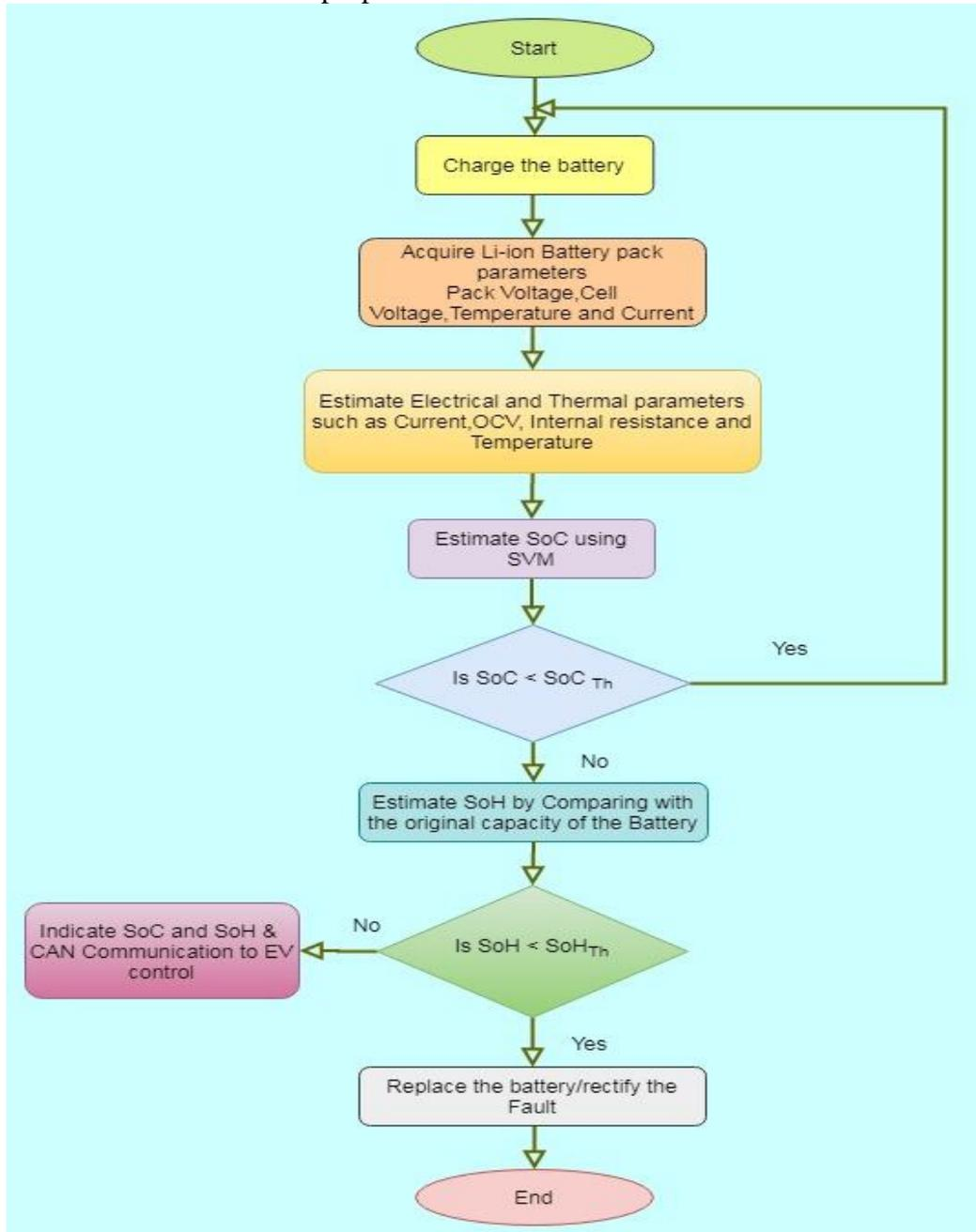
Fig 3.Flowchart of the Proposed Battery Management system
