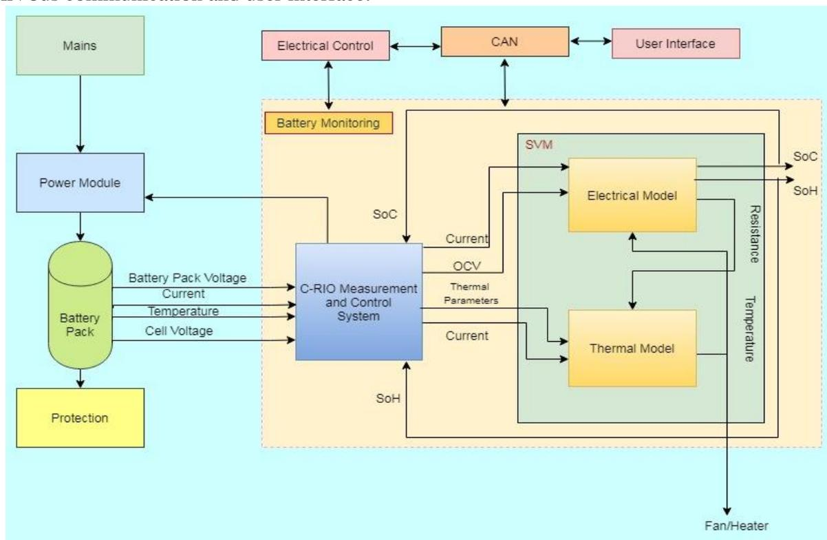
Fig 2. Proposed Battery Management system
