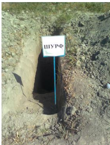
Pic 2.Shurf, a dug for determining Pic 3.Different soil depths the levels of the watershed and soil layers
