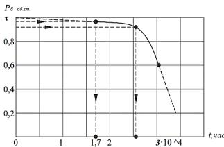
**Fig.2. Dependence of the probability of failure-free operation time of an induction motor of a railway service car**
