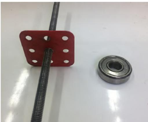
**Connecting the plate to the central spindle rod and the central rod rotary bearings**
